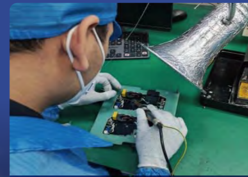
Improvement Before (Manual Soldering Rework)
